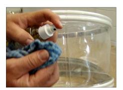
You can also rinse or wash your BFM® connector using non-corrosive detergents in warm water. It is important that the BFM® connector is wiped clean and dry of any residual chemicals after washing, and the internal surfaces of the BFM® spigots are also wiped clean and dry.
