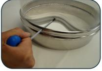
**<u>STEP 1</u>** Insert the removal tool in the opening of the hole and push towards the centre of the fitting.
