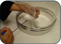
**STEP 2** Hold the seal of the connector and remove from the spigot.
