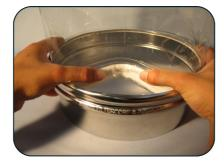
**STEP 2** Seat the back of the connector into the BFM® spigot and release. The cuff will snap into the spigot.
