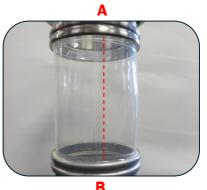
**STEP 3** Snap into the second spigot ensuring that the welded seam of the connector is straight and that points A and B are directly in line.
