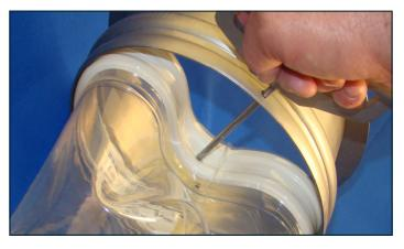
The Snap Ring of the BFM<sup>®</sup> TR connector is manufactured to have a firmer fit than a standard connector. Once a BFM<sup>®</sup> TR connector is fitted, it can only be removed by using a TR Release Tool, which is simply inserted into a 6mm in the side of both the upper and lower spigots.
