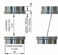
In-line static equipment IG = CL - 10mm(Minimum)
